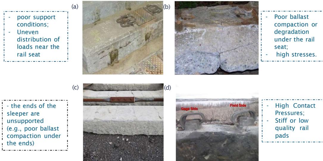
Figure 6. Examples of damages: (a) Horizontal cracks, (b) rail seat positive crack, (c) center negative cracks on concrete ties with abraded bottom, (d) deteriorated rail seat surface, (Lam et al., 2012)
