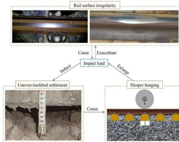
Figure 3. Interaction between a rail surface irregularity and a hanging sleeper. The variations in the width of the shiny running band indicate rail surface irregularity, (Yang F. et al. 2021).
